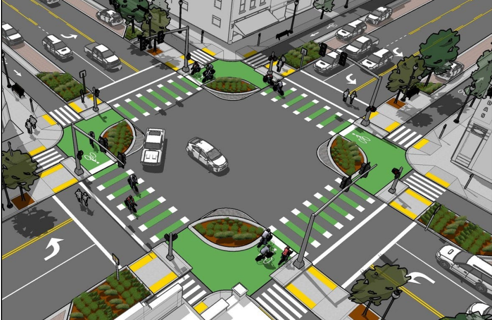
A rendering of bulb-outs at an intersection with protected Class IV bike lanes.
