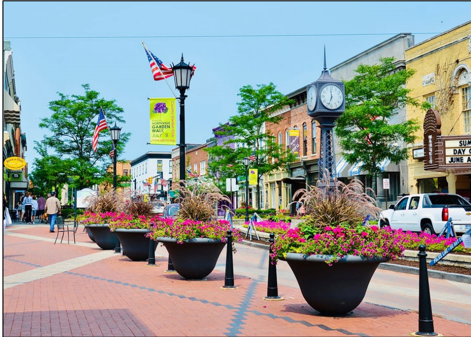
Decorative planters as bollards that fit the aesthetic of a particular corridor.
