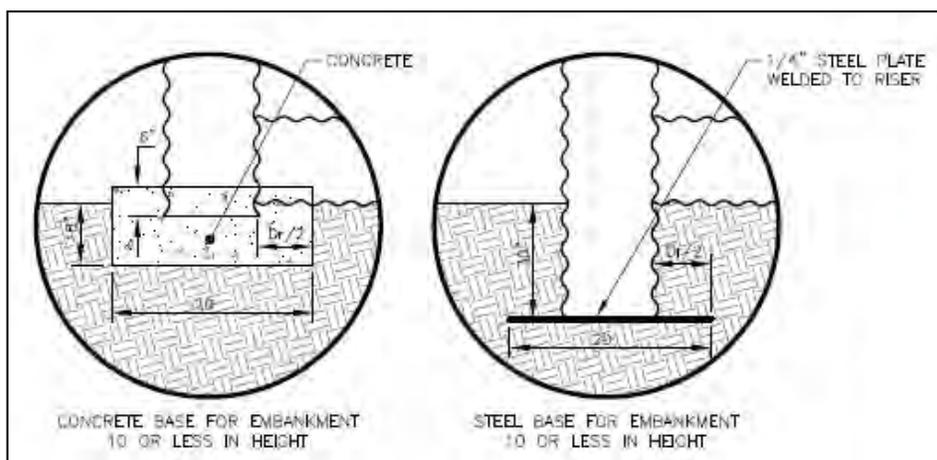
**Figure 7.31-4 Anti-Flotation Device**
