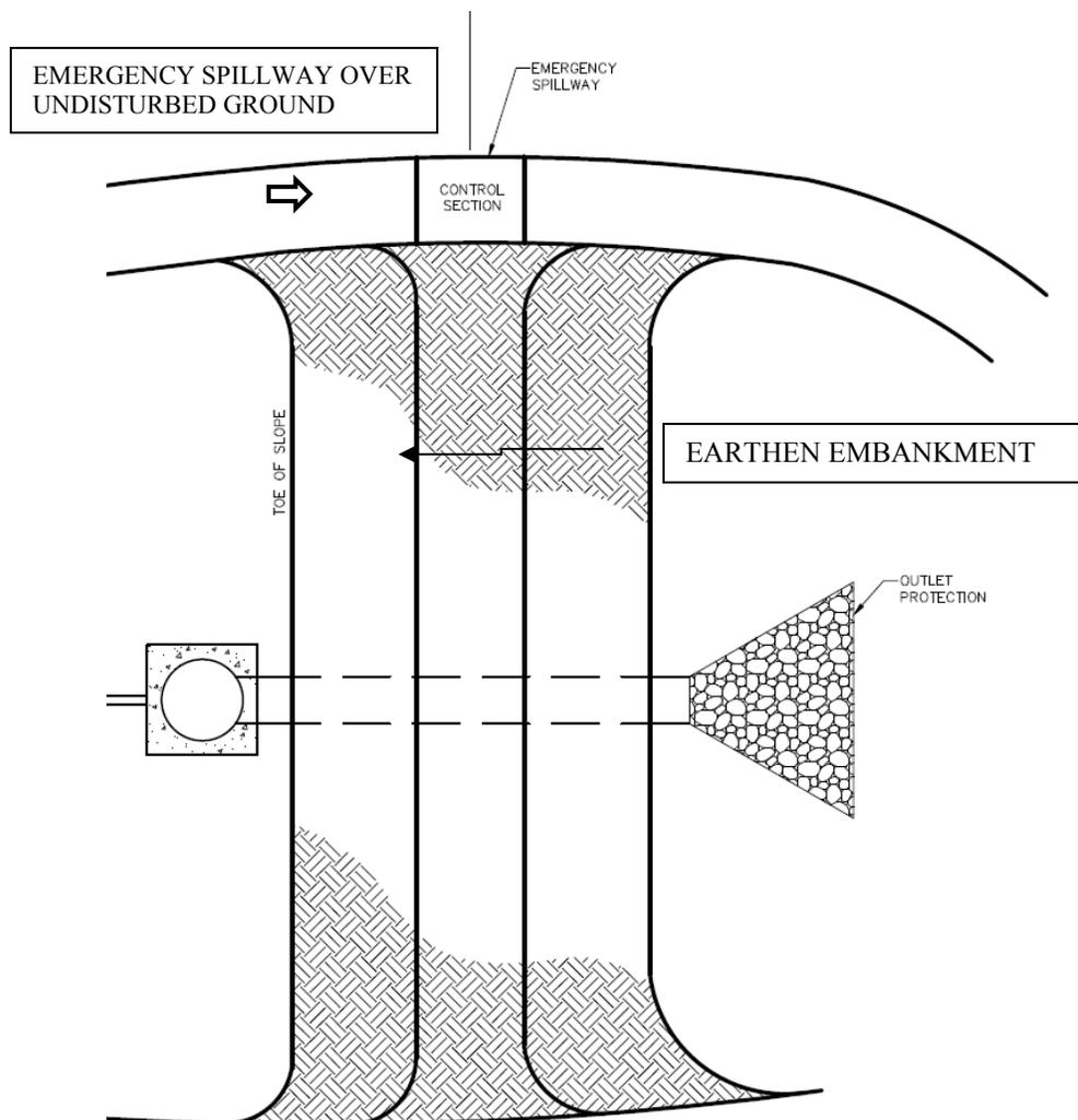
**Figure 7.31-11 Earthen Embankment**
