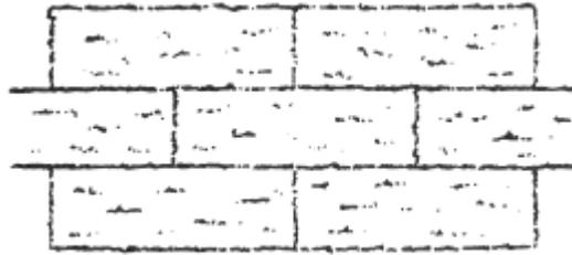
**Figure 7-7.10-1. Correct sod placement**
