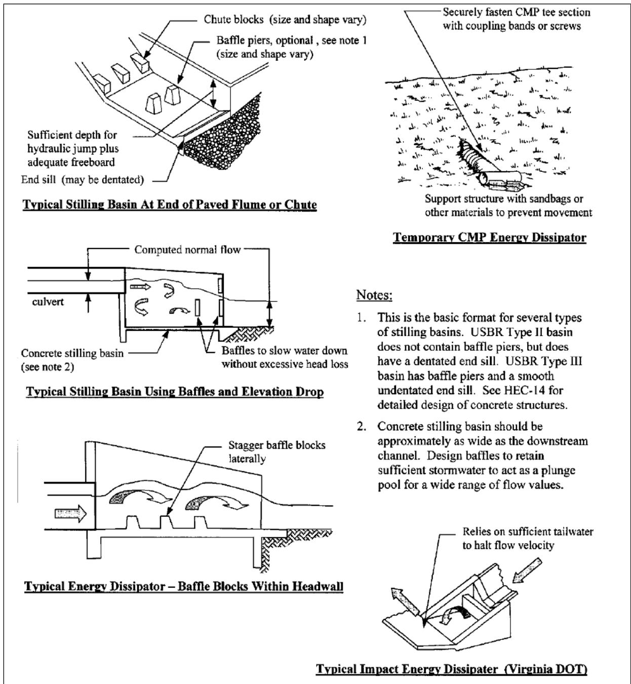
Figure 7.23-2 Stilling basins and other energy dissipaters
