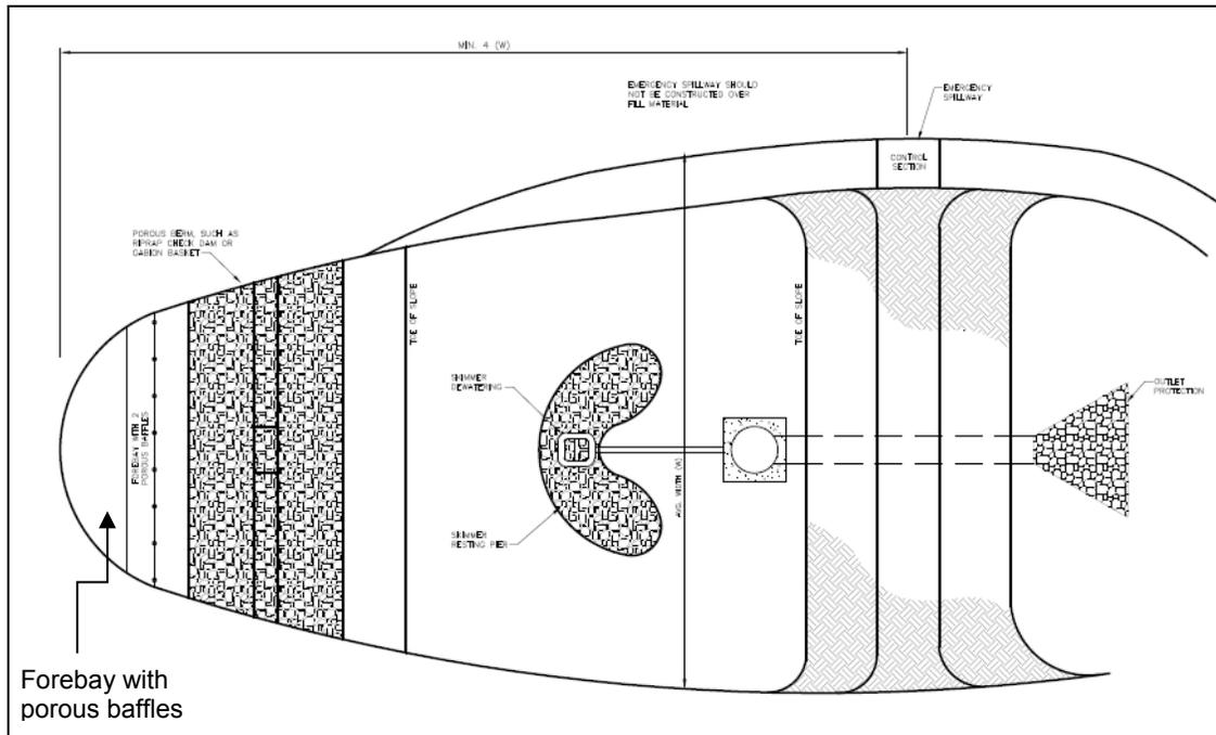
Figure 7.31-2A Sediment Basin with Forebay, Plan View
