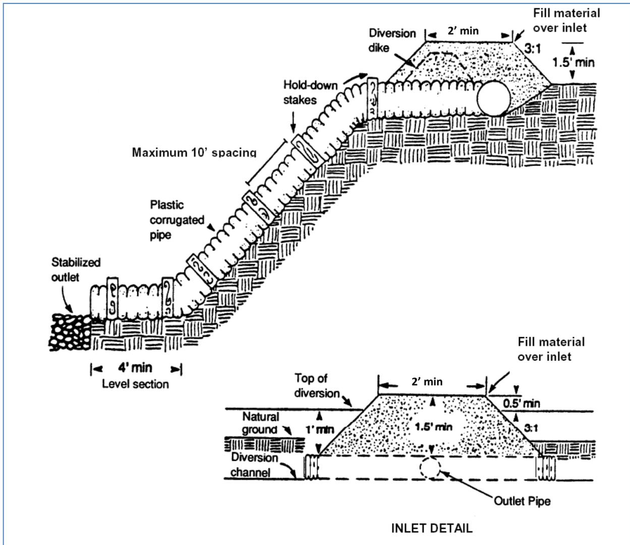
Figure 7.24-1 Slope drain pipe and inlet detail
