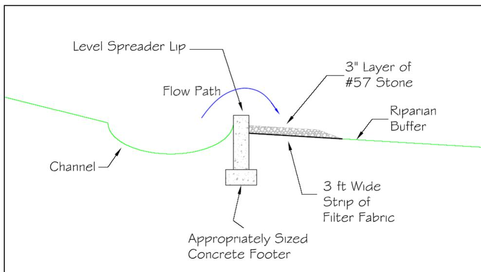
**Figure 7.26-1 Cross Section of Concrete Level Spreader**
