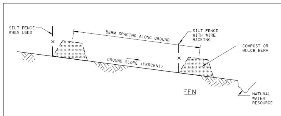
**Figure 7.38-2 Mulch Berm with Silt Fence with Backing**
