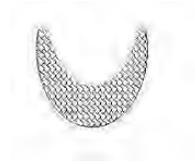
*Filter rings should be part of an overall system of BMPs. Above, the filter ring is providing sediment control while the mulch is providing erosion control.*
