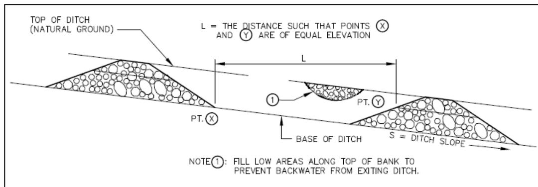
**Figure 7.20-2 Spacing between check dams (Source: TDOT)**
