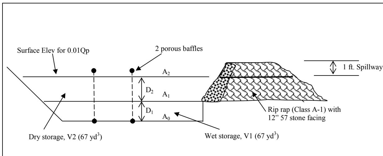
**Figure 7.32-1 Sediment trap**
