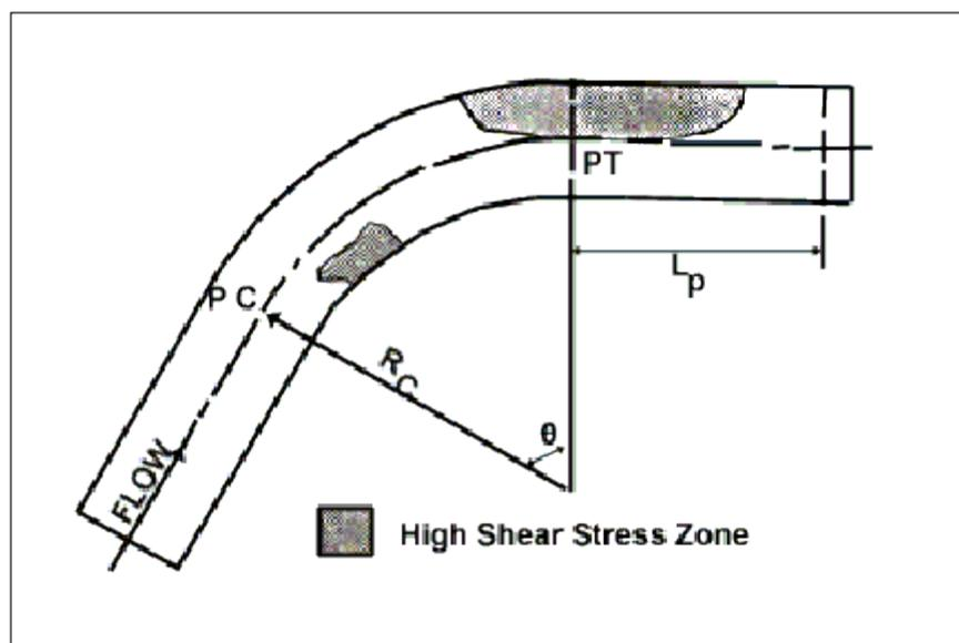
Figure 7.27-3 Shear Stress Distribution in a Channel Bend
