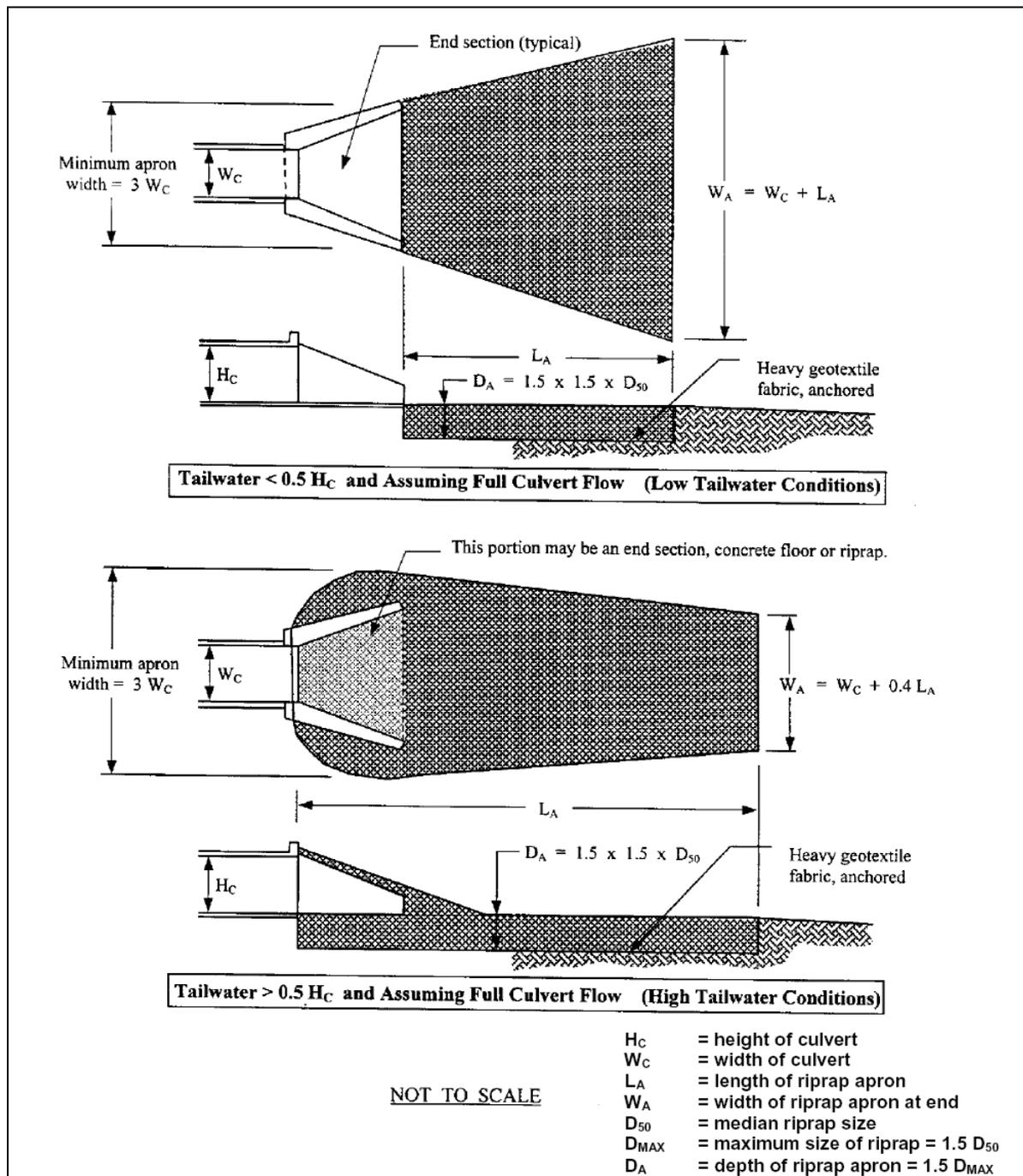
Figure 7.23-1 Riprap outlet protection dimensions
