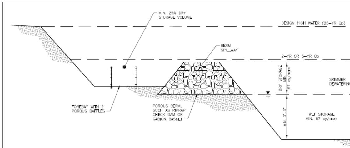
Figure 7.31-2B Cross Sectional View of Forebay, Showing Elevations
