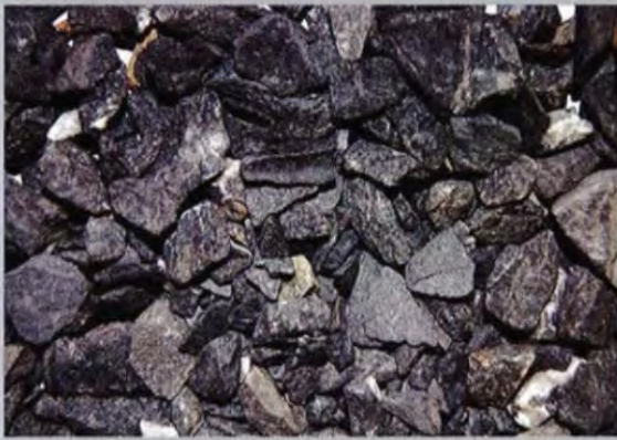
Single Chip Seal Aggregate (irregular size & elongated aggregate)
