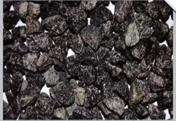
Single Size Cubical Aggregate utilized in High Performance Chip Seal
