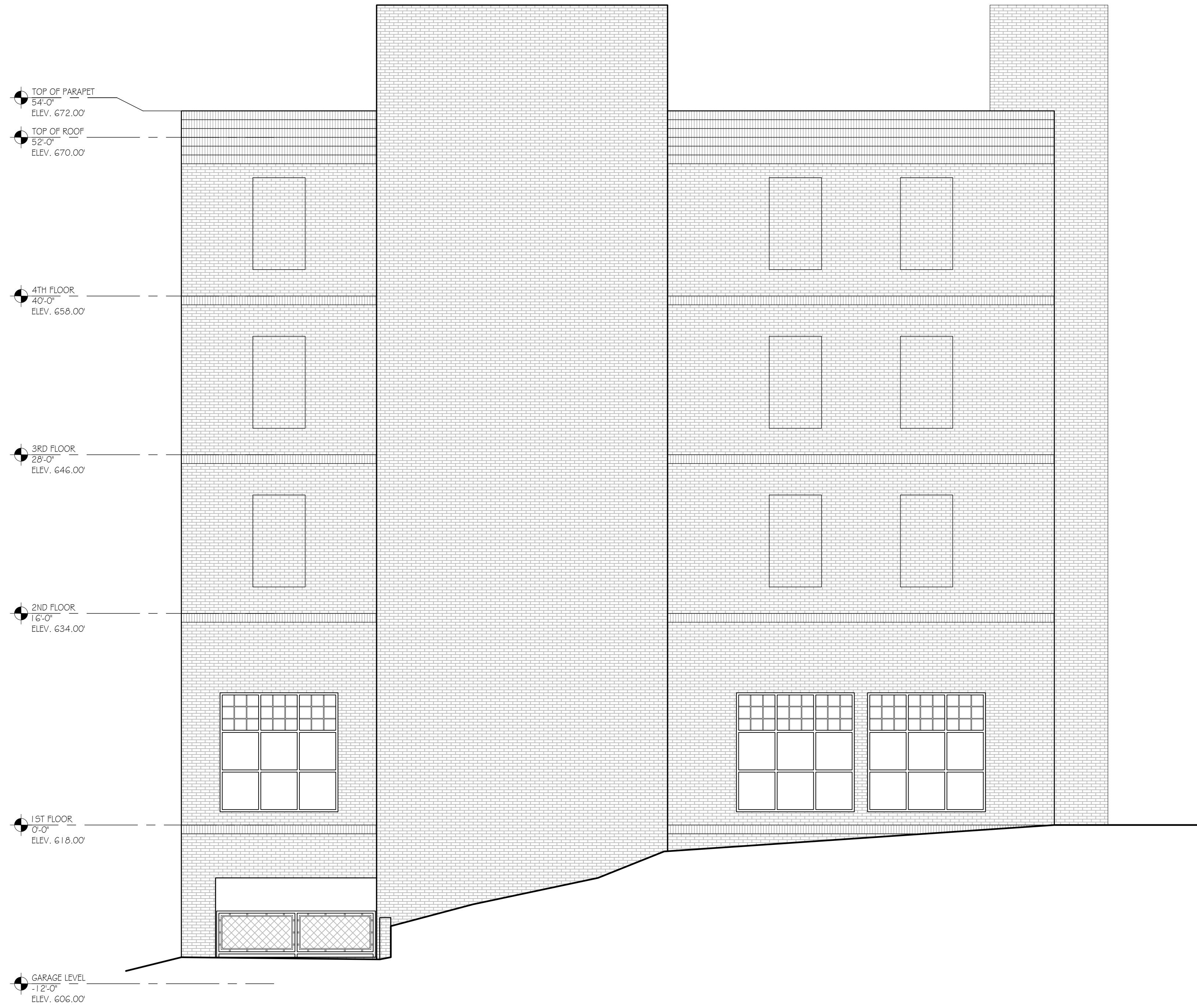
EAST ELEVATION SCALE 3/16" = 1'-0"
