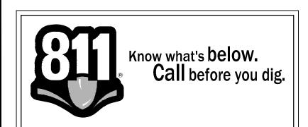
PENNSYLVANIA ACT 287 (1974) AS AMENDED BY PENNSYLVANIA ACT 199 (2004) REQUIRES NO LESS THAN THREE (3) WORKING DAYS AND NO MORE THAN (10) WORKING DAYS NOTICE TO UTILITIES BEFORE YOU EXCAVATE, DRILL, BLAST OR DEMOLISH. PA ONE—CALL SERIAL NO. 20231515029
