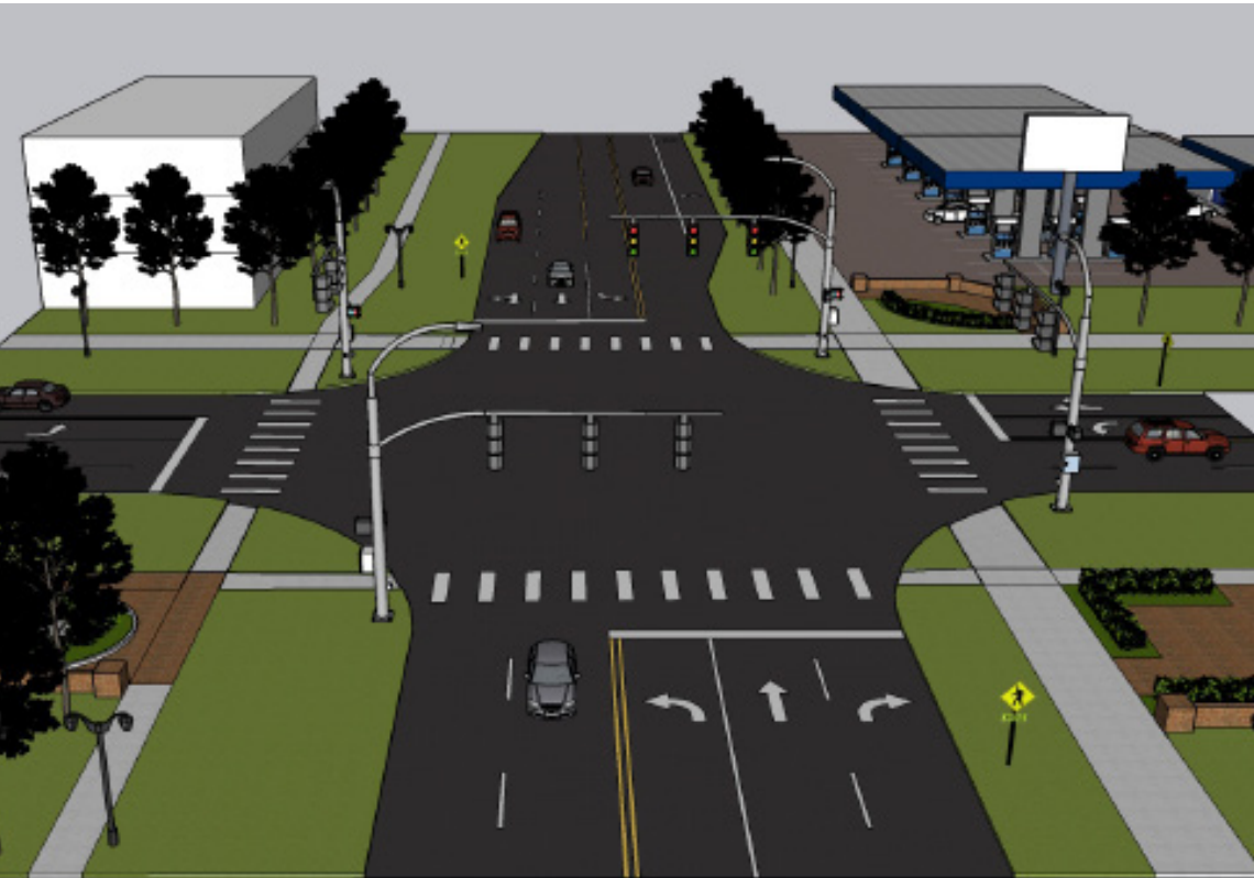
Figure 5-30. Northbound view of Tyler Road intersection with proposed realignment and addition of left-turn phasing Source: Wade Trim
