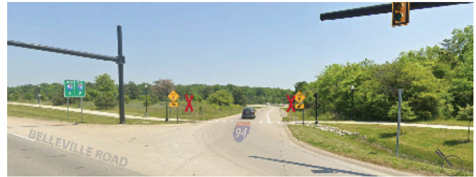
Figure 5-35. Eliminate right turns onto ramp when pedestrians are present Source: Wade Trim
