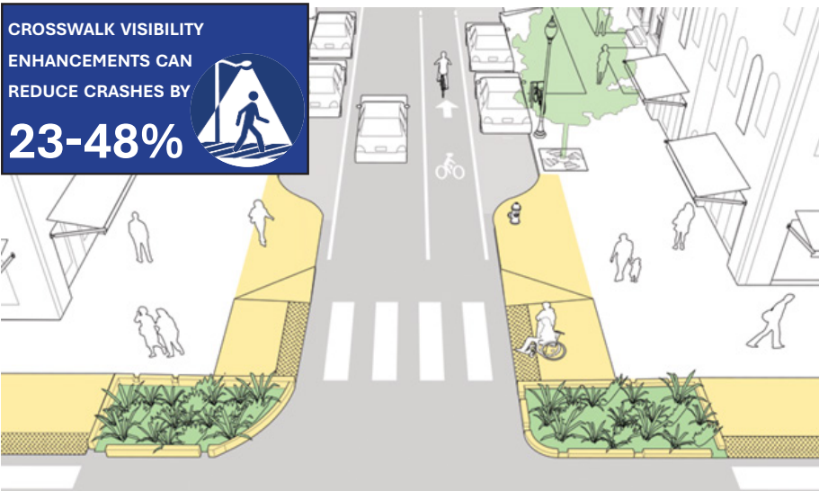
Figure 5-5. Curb extension or bump outs encourage slower speeds and often include decreased turning radii. Source: NACTO Urban Street Design Guide
