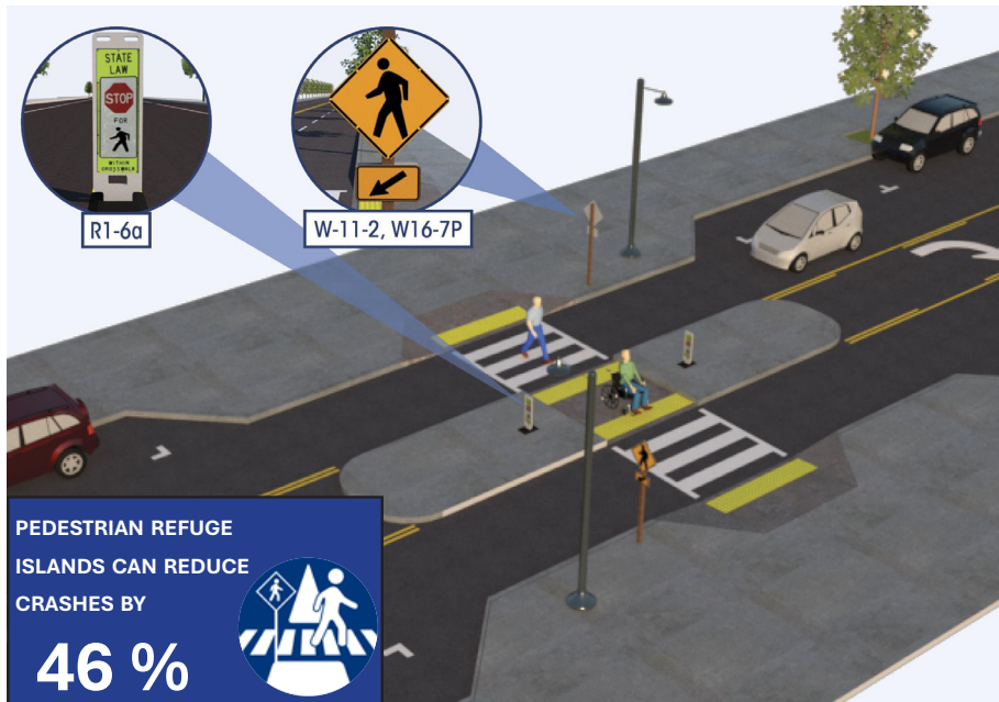
Figure 5-6. Pedestrian refuge island Source: Federal Highway Administration
