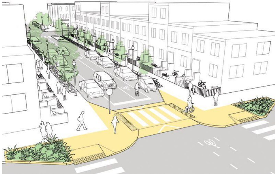
Street design elements for commercial area streets. NACTO Urban Street Design Guide
