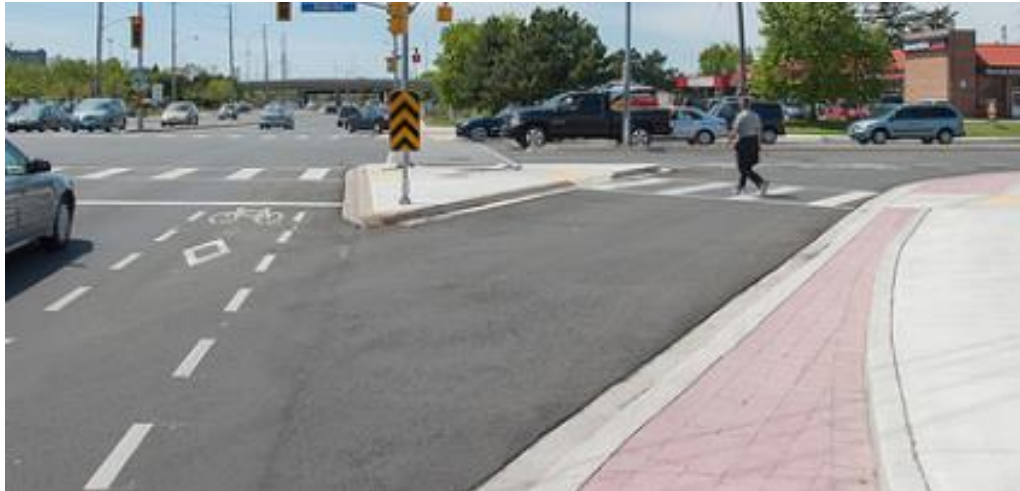
Figure 6-2 – Design Example – Intersections for freight and pedestrians
