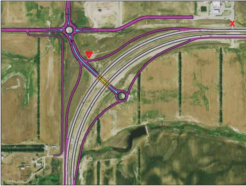
Figure 14C – Option C: Diamond Interchange with Roundabouts
