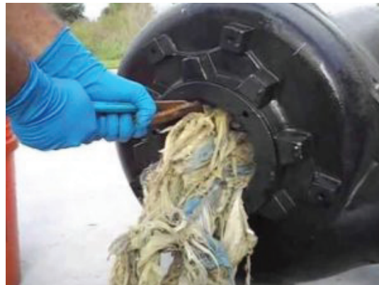
A YCUA wastewater pump, clogged with wipes.
